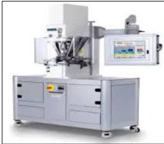
Figure9: Bi-layered tablet press with displacement monitoring
